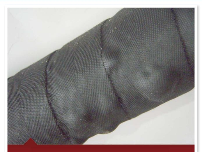
An indication of internal hydraulic hose failure. Hydraulic Hose assemblies having blisters on the outer shell must be replaced immediately.
